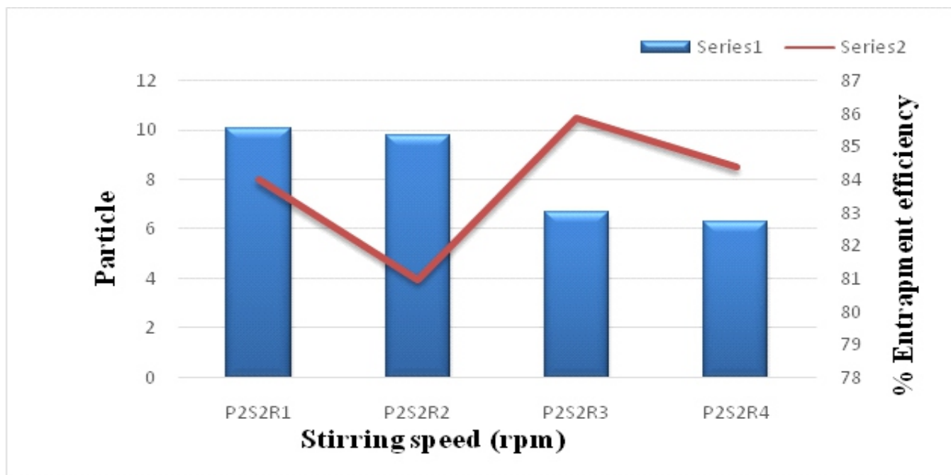
Figure 11. Effect of Stirring speed on particle size and % entrapment efficiency
